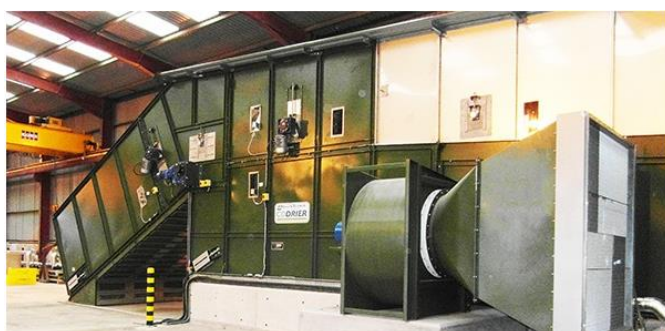
Figure 51. Uist Asco - conveyor dryer, hand harvesting 15,16
